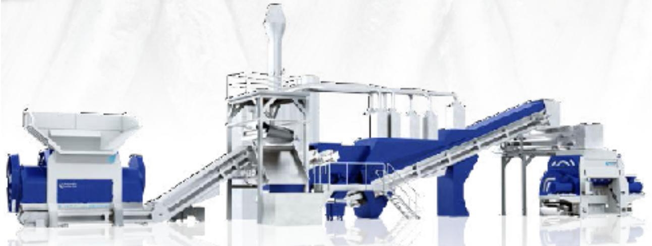
**\*3 Pre-schredder mill** Size differs and to large objects can not be handled in the incinerator. Here we have a shredder that crush all to max 50 cm size. This is what boiler can handle and we see we have a steady flow of this material. Today most materials on a city dump is plastics and burnables and often 70 % of content have a reasonable good energy content when burned.
