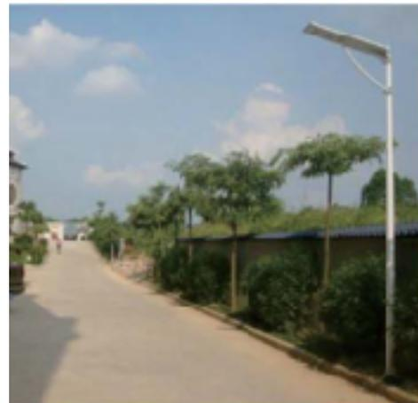
This is a simple to use and simple to install solar lamp with good performance balanced to reasonable costs and Life Cycle Cost. It is designed to operate for 7-10 years with no service and can easily be upgraded for extended life when needed.
