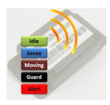
This is a tag with a very efficient micro controller inside that can be set to measure and calculate and work as a small PLC system stand alone. The integrated battery is OK for 10-15 years if communication is not to large. Here we can interface almost anything and calculate and analyse in tag and then send formation if needed.
