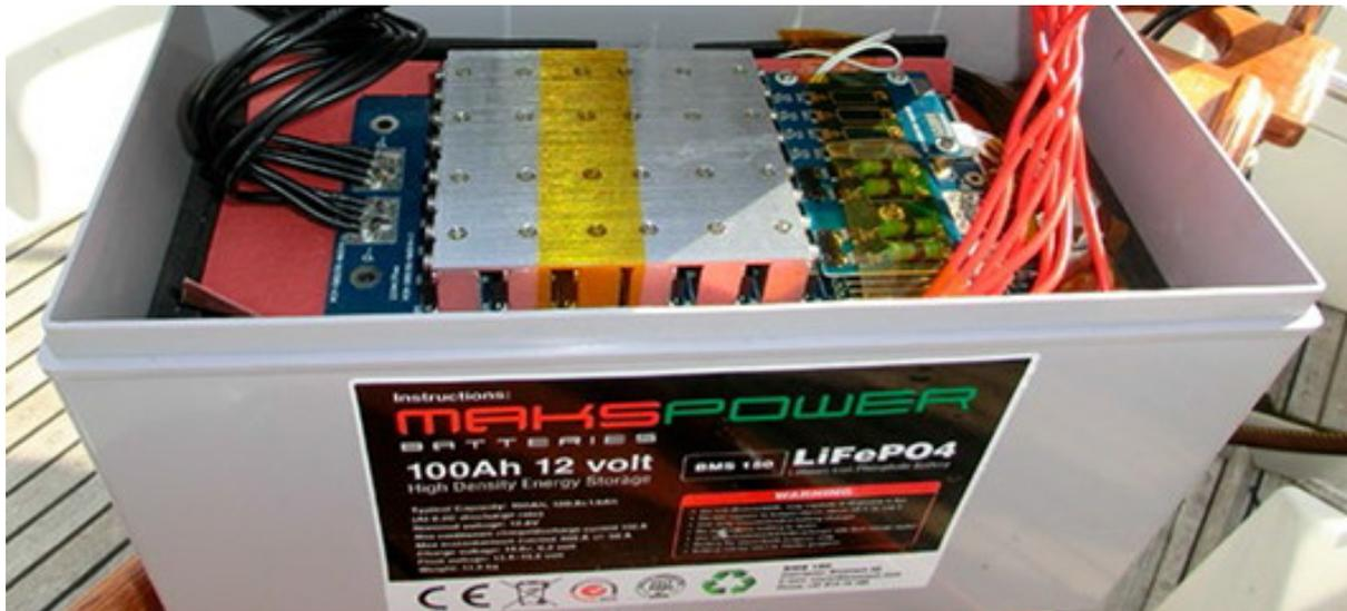
Battery box have BMS battery management systems inside the sealed unit. This makes battery to act like a lead battery so exchange is very simple in old system as all works directly. BMS system control and protect battery to damage and bad handling. The +85C operation makes battery very good in warm areas where other battery units will suffer hard. Other lithium battery are often rated max 60C so this is much better. Solar lamps are a very hot place where this can be the solution.
