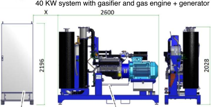
40 KW system with gasifier and gas engine + generator
