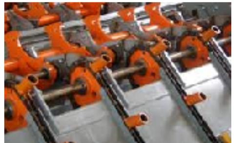
**Section 1.** Log table with separator. Logs are normally put on a table by a tractor with a gripper system. Here a separation unit sort out logs 1 by one and they are stored in a stand by position close to the lock door. Number of logs here is controlled and is preset. System is automatic and needs only the tractor driver to supply wood pieces. Alarm unit can send a signal by radio to tractor when magazine is getting empty.
