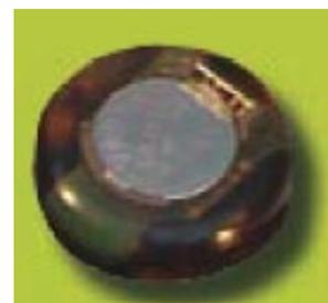
Waterproof mini tag. This is ideal to add somewhere in the cloths and het invisible for the alarm sensors. The battery live for about 1 year and is easy to replace
