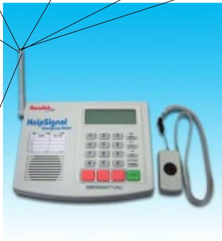
Small central unit with Telephone interface. This can control several zones in a building and several functions and alarms
