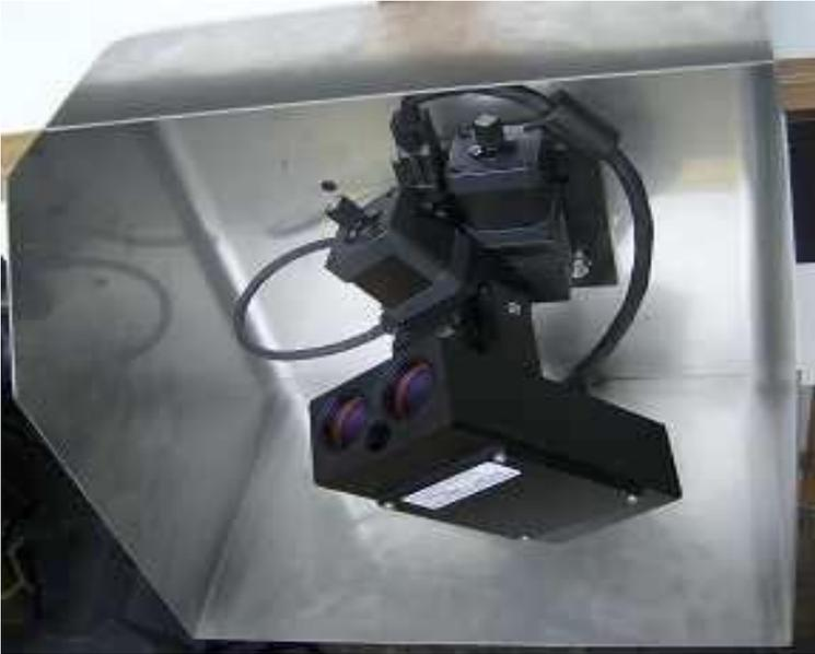
Ladar unit is based on a 2 axis laser scanner with a high speed and high accuracy distance meter.
